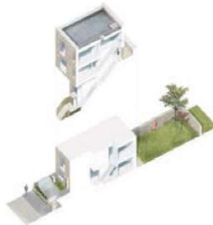
Fig 103 Stacked maisonettes - the reinvention of this post-war format is being used as way of increasing the density of the typical terraced street typology (Allies and Morrison)
